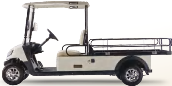
·Shuttle 2 cargo deck Cargo deck size: 1735*1160*350mm
