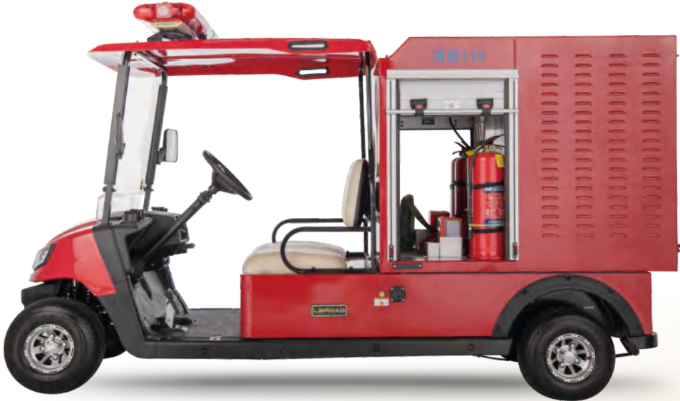
•Firefighting Car (without water tank)
