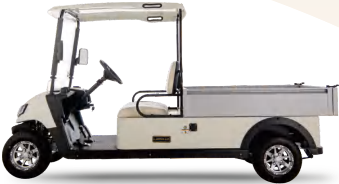
·Shuttle 2 Aluminum cargo box Aluminum cargo box size: 1478*1145*270mm
